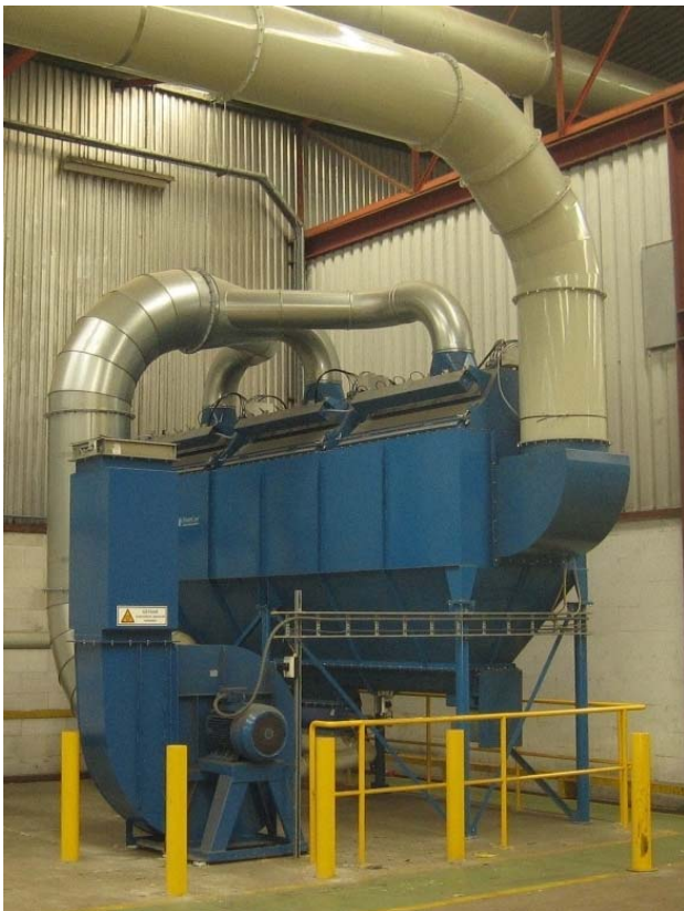
PowerCore® CPC-unit with a capacity of 20.000 m 3 /h
