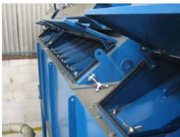
PowerCore® CPC-unit with a capacity of 20.000 m 3 /h
